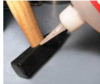
Flying off the handle is never good, particularly if it's a hammer head. The traditional way to tighten a loose hammer head is a bit of work, but there's a fast and easy solution available for about 50 cents - superglue. Simply put a couple drops in from the handle side, let it set up, and then a few drops from the top side. Be sure to get the thin superglue, not gel. It penetrates better. Packages of two superglues are usually available at the 99 cent store.
